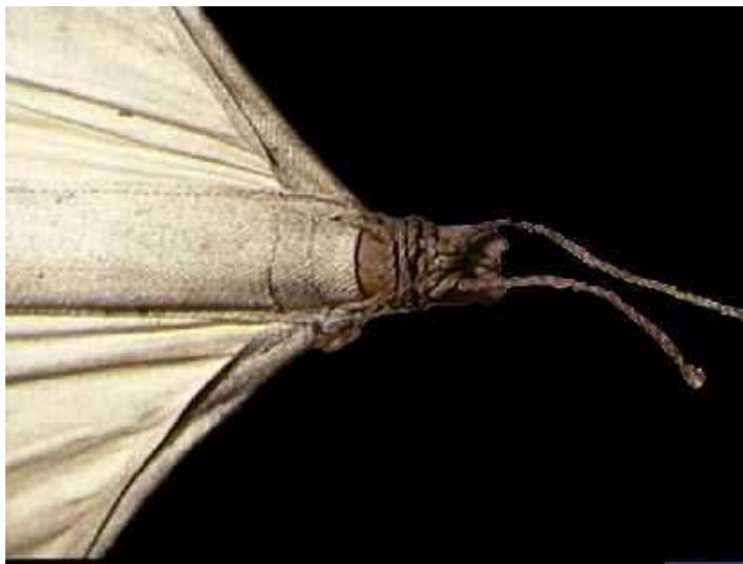
Fig. 18: Mounting of sail spars
