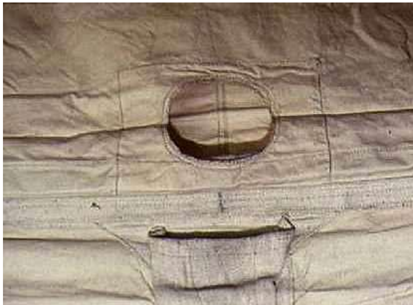
Fig. 12. Hole for diagonal spar with pocket
