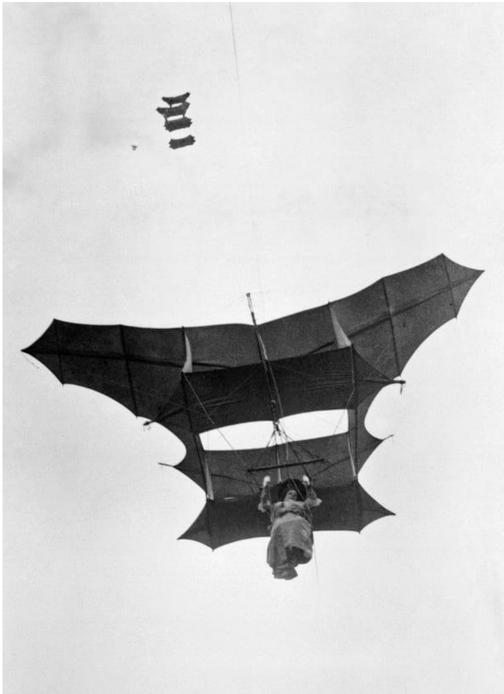
A passenger flying Man-lifter War Kite designed by Samuel Franklin Cody. (Royal Engineers official photographer) The Hafner Rotachute
