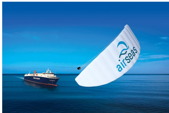
AirSeas announced the installation of the first automated kite propulsion system on a commercial vessel.
