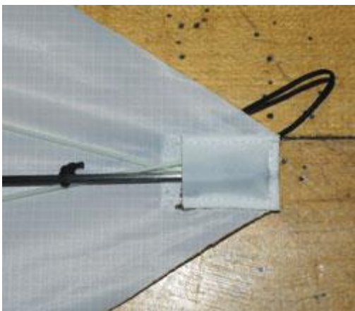
The tail of the bird with a pocket for the middle stick Stick pocket for the wings including openings in the sail for the head stick Corresponding to the stick pocket on the head Pockets in the next
