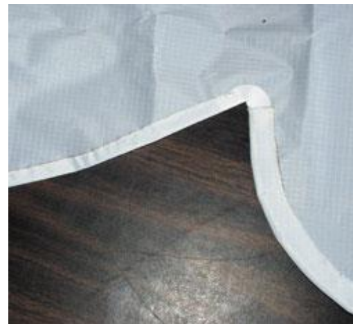
Reinforcements in the wing area
