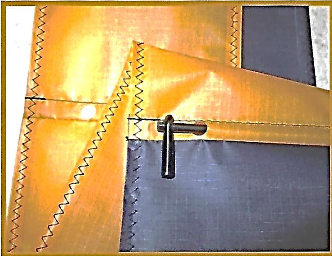
Pic 14. Spar sticking out of hole with end cap fitted onto spar.
