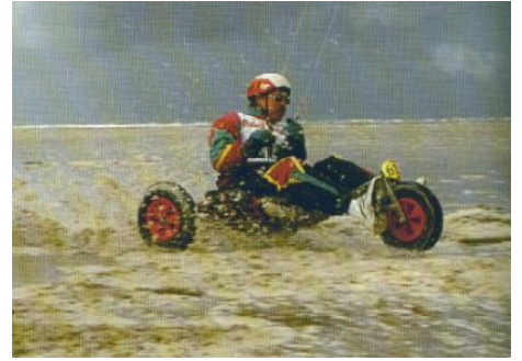
New Zealand: Peter Lynn also designed a modern kite "buggy" made from stainless steel and powered by large maneuverable kites. George Pocock used the same idea in England in 1822.
