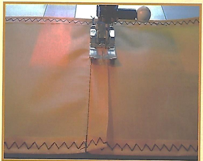
Pic 10. Sewing the spar channel close to the edge.
